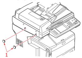
(i) Using the tool provided (2), lock the scanner at the two locations as shown.
